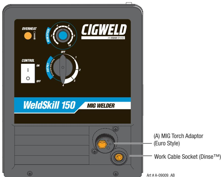
Figure 3-5 Attaching Mig Torch
