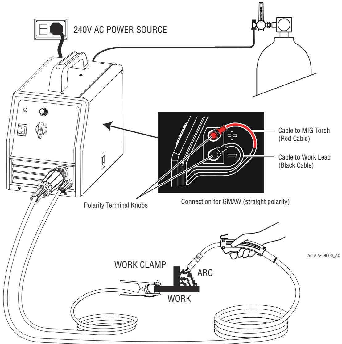
Figure 3-17: Gas Shielded Set-up for WeldSkill 150 Mig
