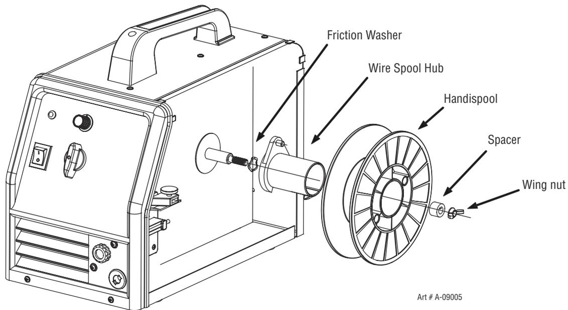
Figure 3-10 200mm Spool Installation
