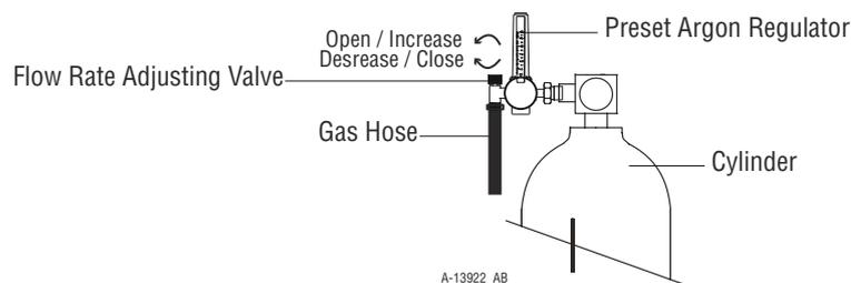
Figure 3-4 Adjust Flow Rate
