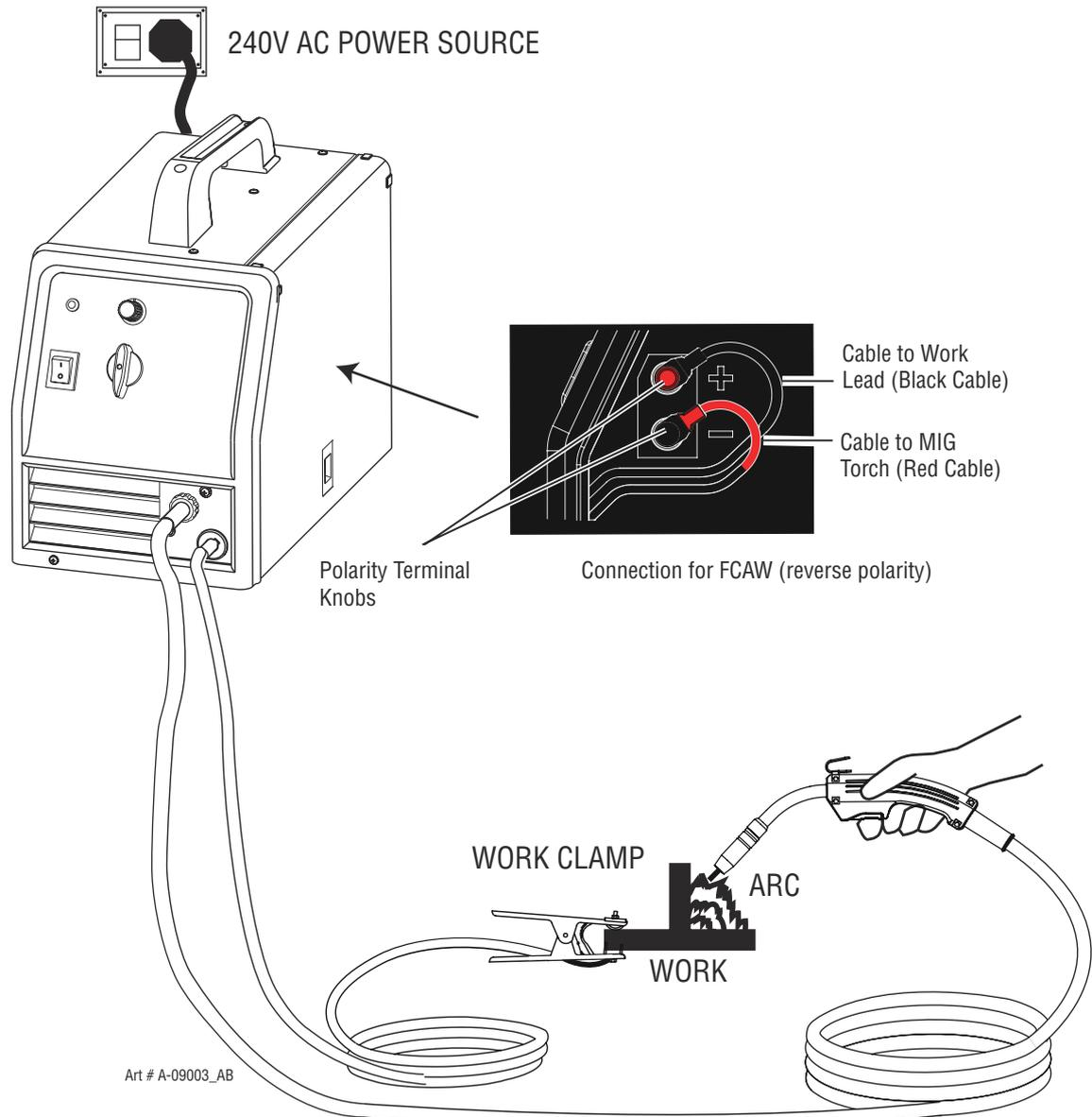
Figure 3-14: Gasless Set-up for WeldSkill 135 MIG
