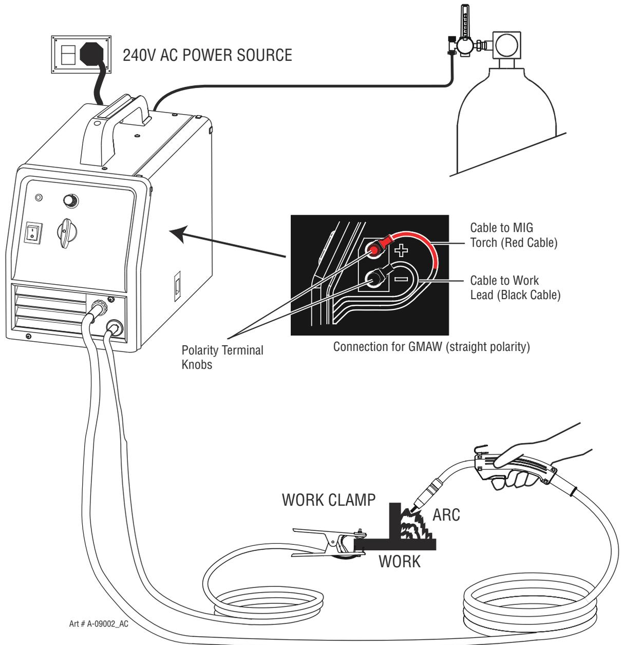
Figure 3-15: Gas Shielded Set-up for WeldSkill 135 Mig
