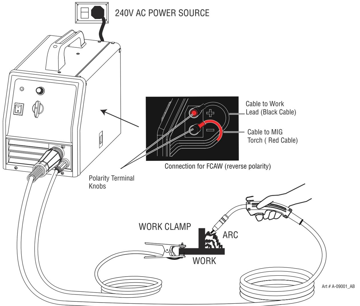
Figure 3-16: Gasless Set-up for WeldSkill 150 Mig
