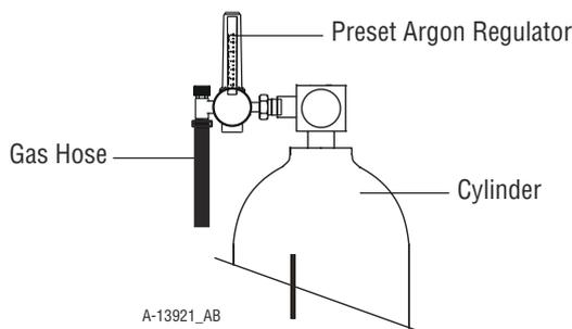
Figure 3-3 Fit Regulator to Cylinder
