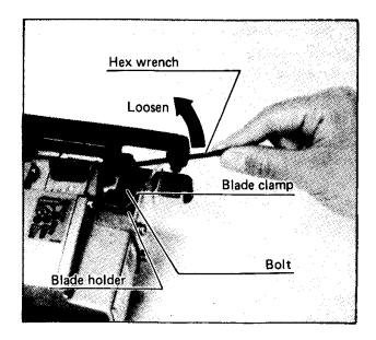
With the blade teeth facing forward, insert the blade into the blade holder as far as it will go.
