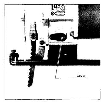
Position 0 — For cutting in soft steel, stainless steel and plastics.
