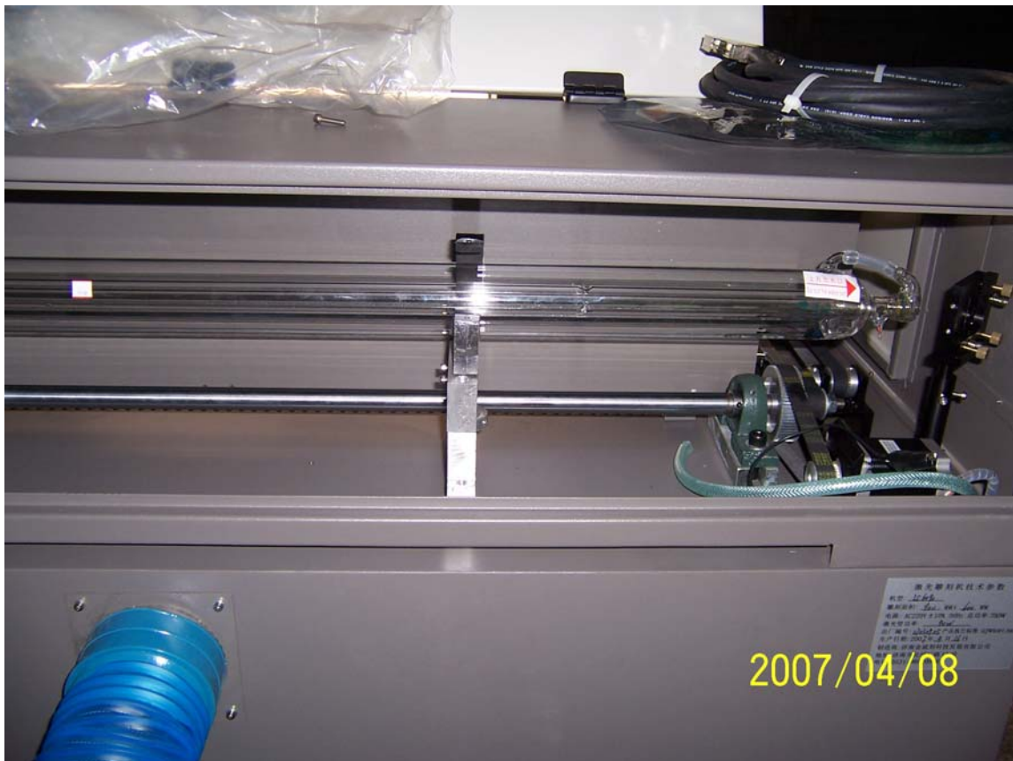
Attention: Light outlet is on the right. Fix the laser tube.
