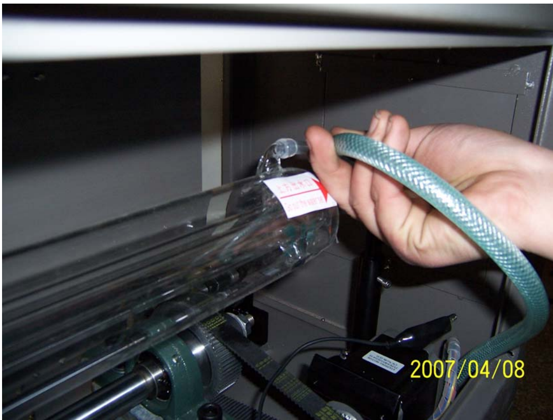
plug in water inlet and outlet.
