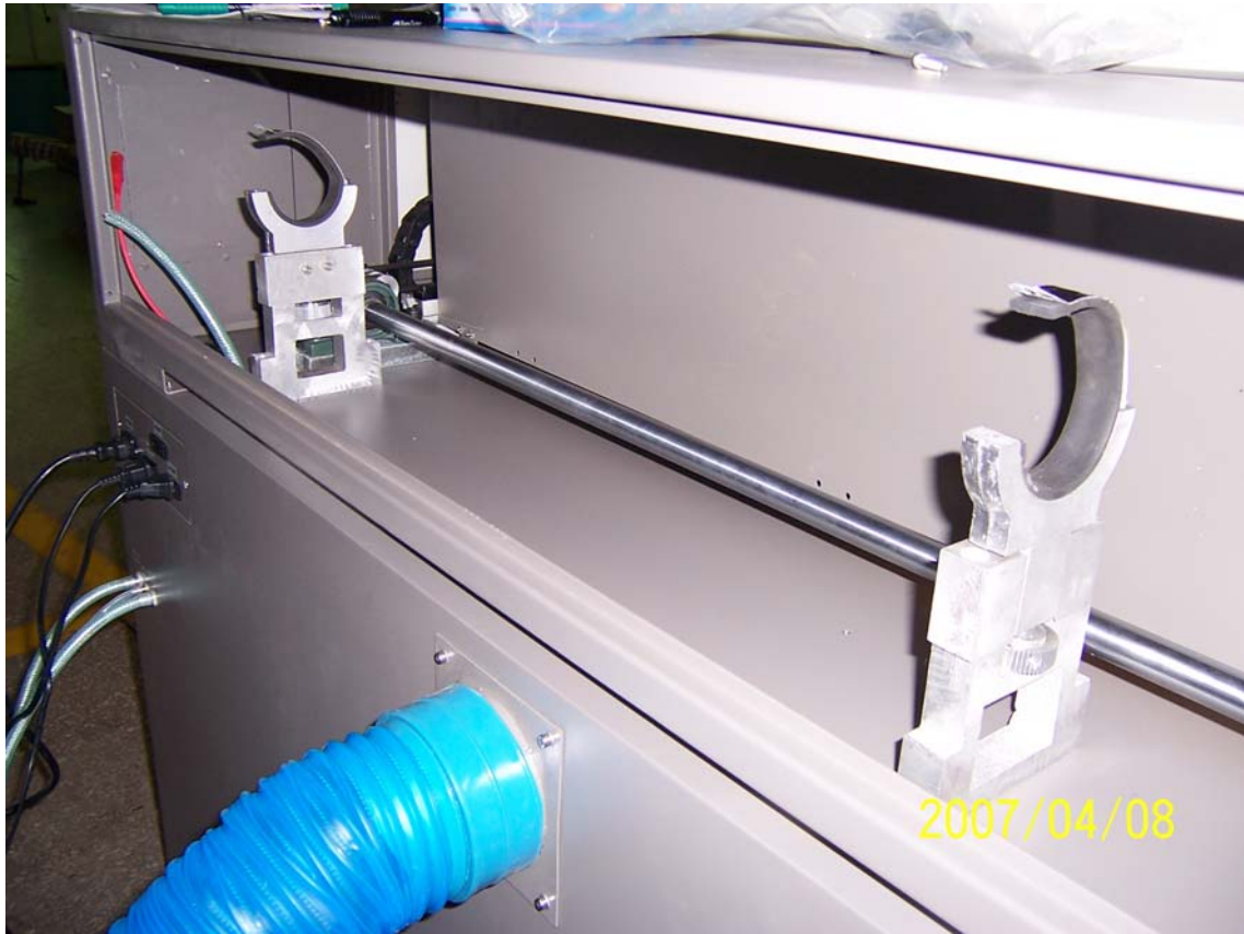
Put the laser tube on two bases.
